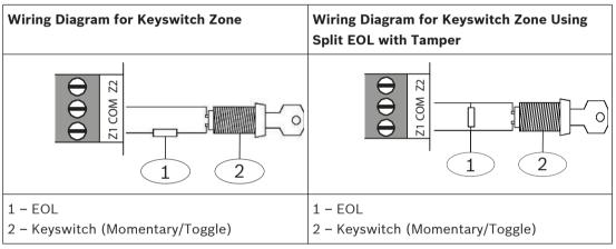
Table 13.2: Wiring Diagram for Keyswitch Zone
